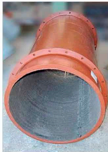
Pipe armored with KALMETALL-W 100 installed in a dust collecting system; inside diameter 400 mm, system thickness 8 + 5 mm
