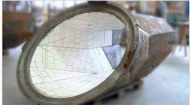
Octagonal hopper in a steel plant; the 50 mm thick KALOCER tiles have been three-dimensionally shaped and cut
