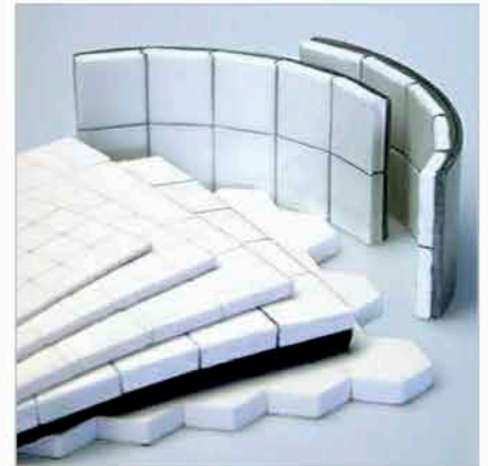
Kalenborn offers KALOCER mosaics in different sizes: square, hexagonal or special design from 1.5 mm to 12 mm thickness. Mosaics can be supplied with book ends. Vulcanized solutions are available.
