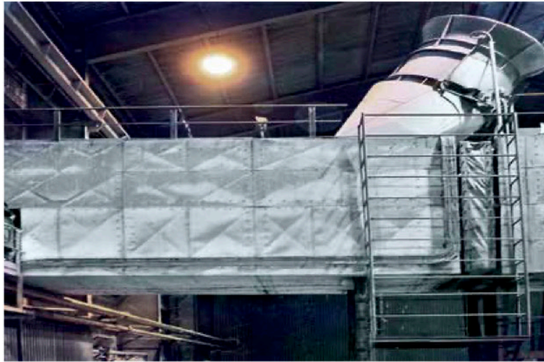
Protection of raw meal pipes against abrasive wear with hard compound KALCRET, lining thickness 25 - 40 mm, operating temperature 200 °C / 392 °F
