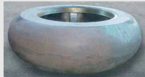
Kalenborn supplies grinding rolls, grinding tables and mill linings for grinding plant used for raw material, coal and clinker. Top: regeneration of a grinding roll with KALMETALL W100, bottom: newly cast component made of KALCAST C153 hard casting, each 1,500 mm Ø.
