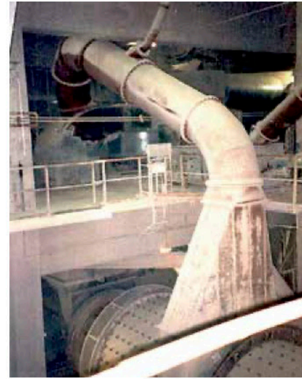
ABRESIST used for the center discharge duct of a ball mill
